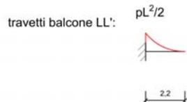
$$q_{\text{bal}} := (0.5\text{m}) \cdot (G_{1\_bal} + G_{2\_bal} + Q_{2\_bal}) = 4.142 \cdot \frac{\text{kN}}{\text{m}}$$
